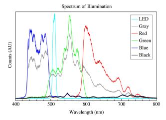
Fig. 4. The illumination spectrum as measured on the sample stage. The LED is a high-power cyan LED through a  $510 \pm 10$  nm filter, the projector was set to project a solid screen of red (RGB[50,0,0]), green (RGB[0,50,0]), blue (RGB[0,0,50]), black (RGB[0,0,0]), or gray (RGB[50,50,50]).
