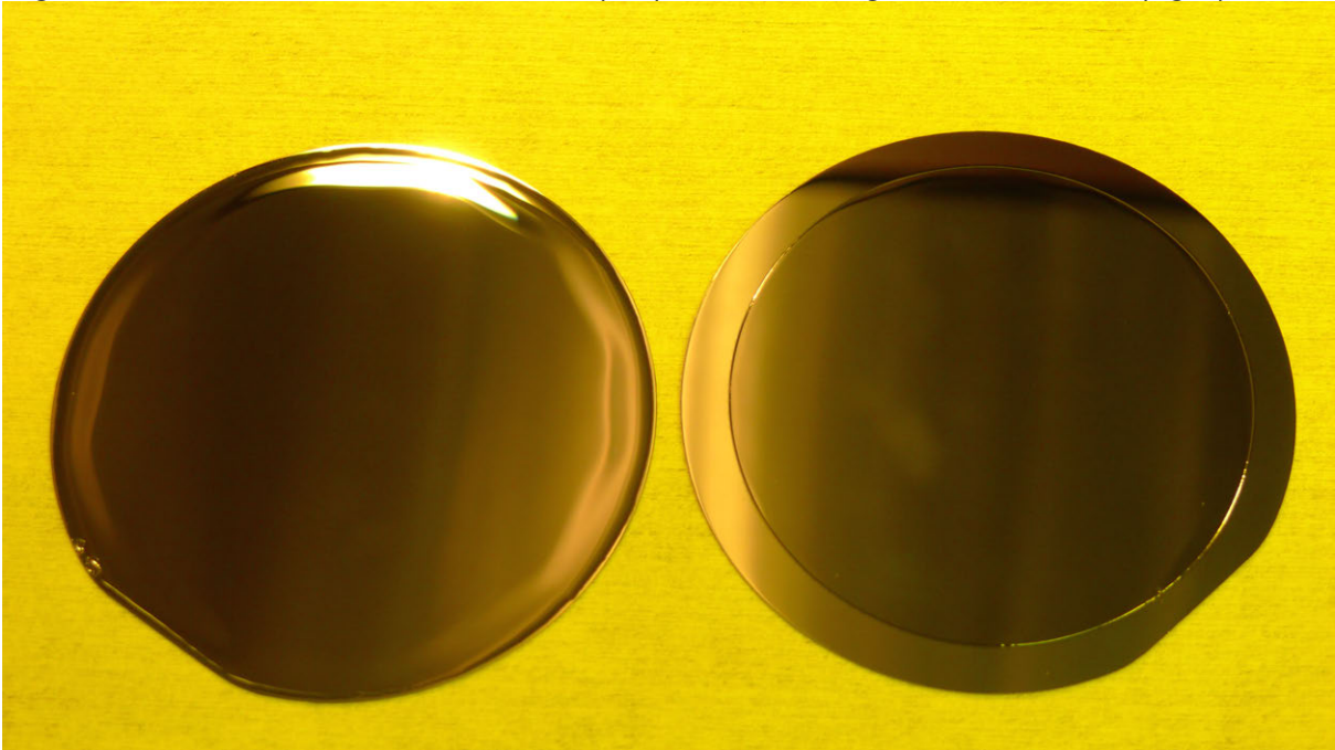
Figure 2: SU8 coated 3" wafer before (left) and after edge bead removal (right).
