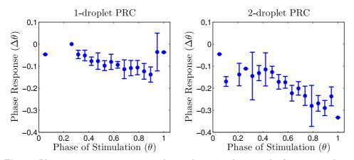
Fig. 4. Phase response curve to perturbation by an oxidation spike from one and two droplets. The spike results in diffusion of  $Br_2$ , which is converted to inhibitor and thus delays the phase. Approximately 10 measurements were performed for data points with  $0.3 < \theta < 0.95$ . Error bars mark one standard deviation above and below the mean phase response.
