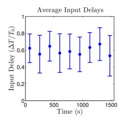
Fig. 5. Average amount of time until an input spikes after light is removed, normalized by the natural period, as a function of time since the start of the experiment. The delay stays relatively constant throughout the experiment. Approximately 20 measurements were performed for each data point. Error bars mark one standard deviation above and below the mean phase response.
